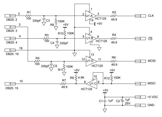
Figure 5.4 Logic level shifting and conditioning circuit
