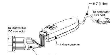
Figure 4.3 MD-CC300-001 communications converter cable
