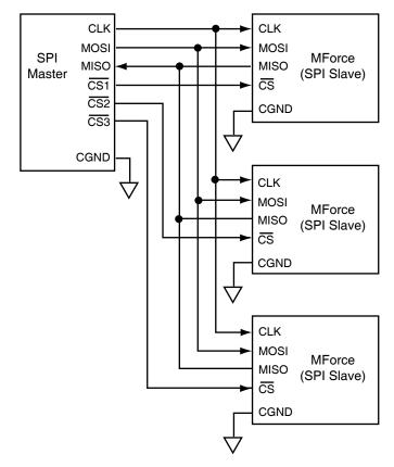
Figure 5.2 Single SPI master - Independent MForce slaves
