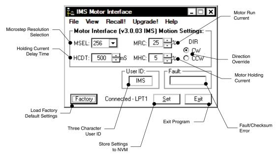
Figure 5.9: SPI Motor Interface motion settings screen
