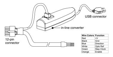
Figure 4.3 MD-CC303-001 USB to SPI converter cable
