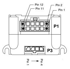
'Figure 4.1 Connector orientation
