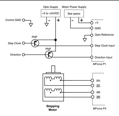
Figure 7.2 Minimum connections, open-collector sourcing configuration
