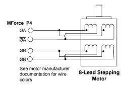
Figure 4.5 8-lead parallel connection
