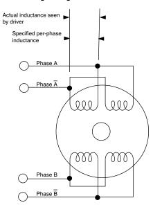
A: 8 lead stepping motor series configuration
