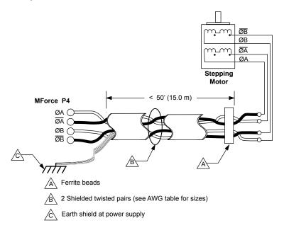
Figure 4.2 Motor cabling under 50' (15.0 m)
