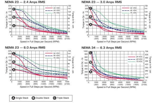
Figure 2.2 Speed-torque curves
