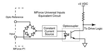
Figure 6.1 Universal optically isolated input equivalent circuit
