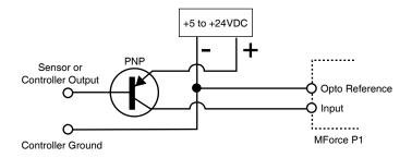
Figure 6.5 Open collector sourcing input
