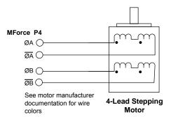
Figure 4.8 4-lead motor connection
