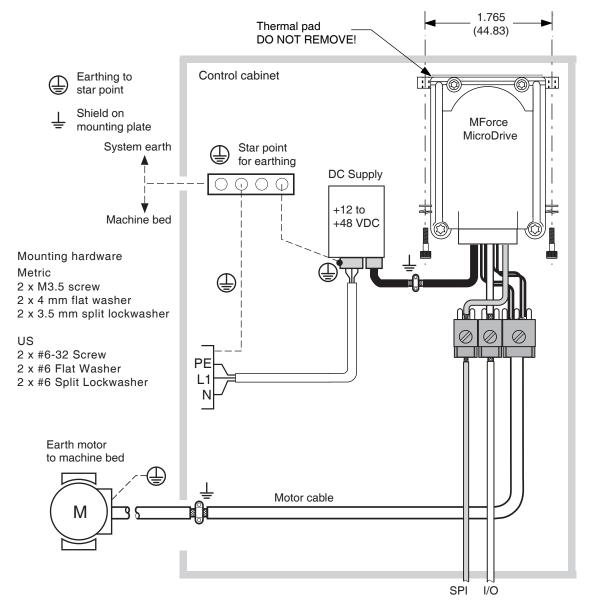
Figure 3.1 MForce Microstepping mounting and cabinet layout
