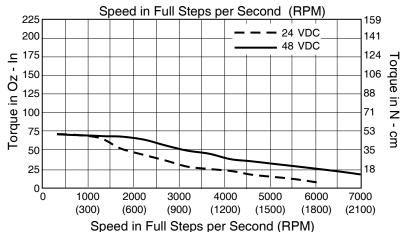
Figure 2.5 Single length NEMA 23 motor
