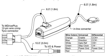
Figure 4.4 MD-CC303-001 communications converter cable
