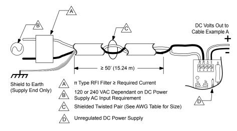
Figure 3.3 50' (15.24 m) or greater, AC power to DC supply
