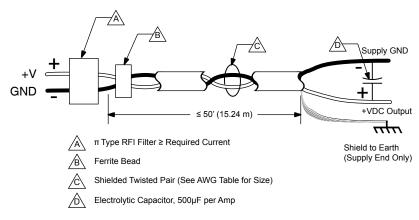
Figure 3.1 DC power supply cabling under 50' (15.24 m)
