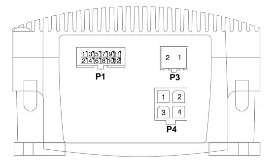
Figure 4.1 Connector orientation
