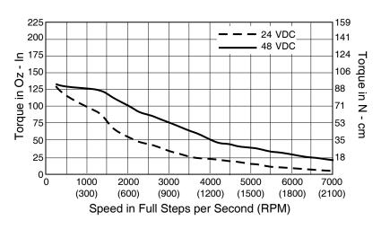
Figure 2.6 Double length NEMA 23 motor
