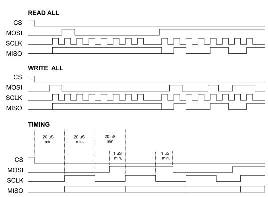
Figure 5.5 SPI Timing
