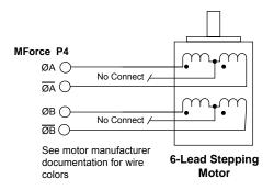
Figure 4.7 6-lead motor full coil configuration
