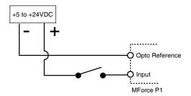
Figure 6.7 Switch interface sourcing input
