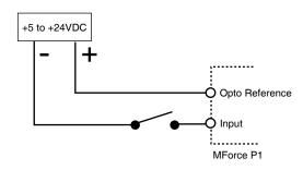
Figure 6.6 Switch interface sinking input
