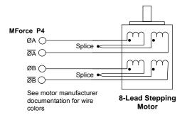
Figure 4.4 8-lead motor series connection
