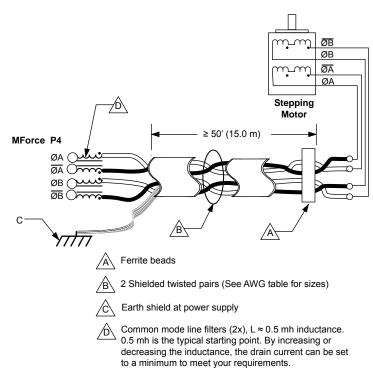
Figure 4.3 Motor cabling over 50' (15.0 m)
