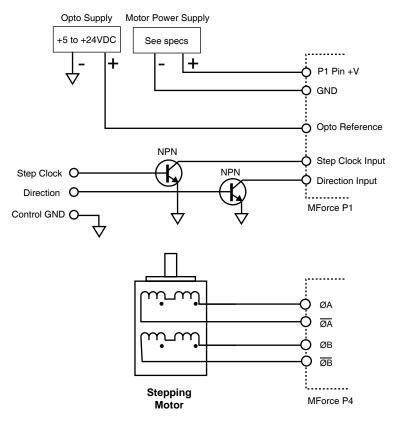
Figure 7.1 Minimum connections, open-collector sinking configuration
