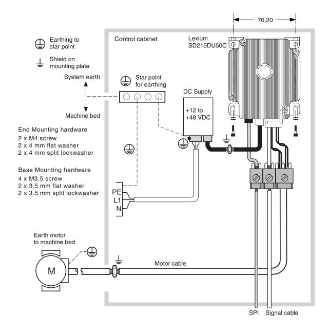
Figure 3.1 MForce PowerDrive Microstepping mounting
