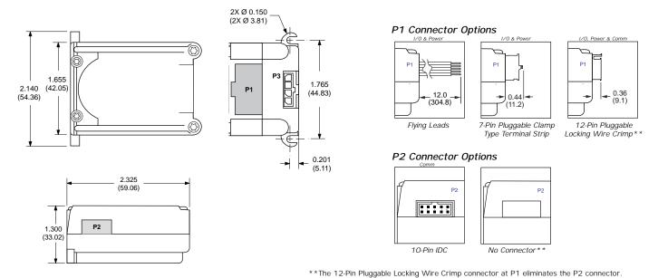
Figure 2.1 MForce MicroDrive Mechanical Specifications
