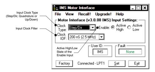
Figure 5.10: SPI Motor Interface I/O settings screen
