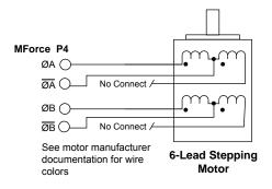
Figure 4.6 6-lead half coil configuration
