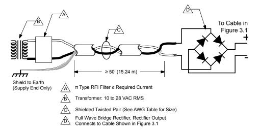
Figure 3.2 50' (15.24 m) or greater, AC power to full wave bridge
