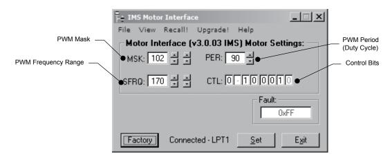
Figure 5.12: SPI Motor Interface PWM settings
