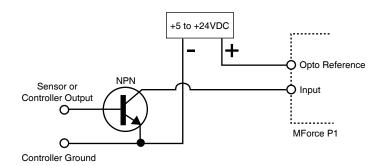
Figure 6.4 Open collector sinking input
